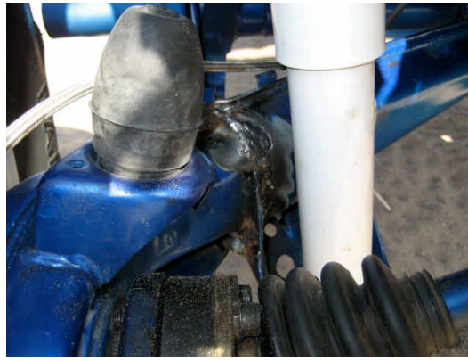
A TORN TRAILING ARM DOESN'T STOP AN INLAND EMPIRE RIDE FOR LONG.
